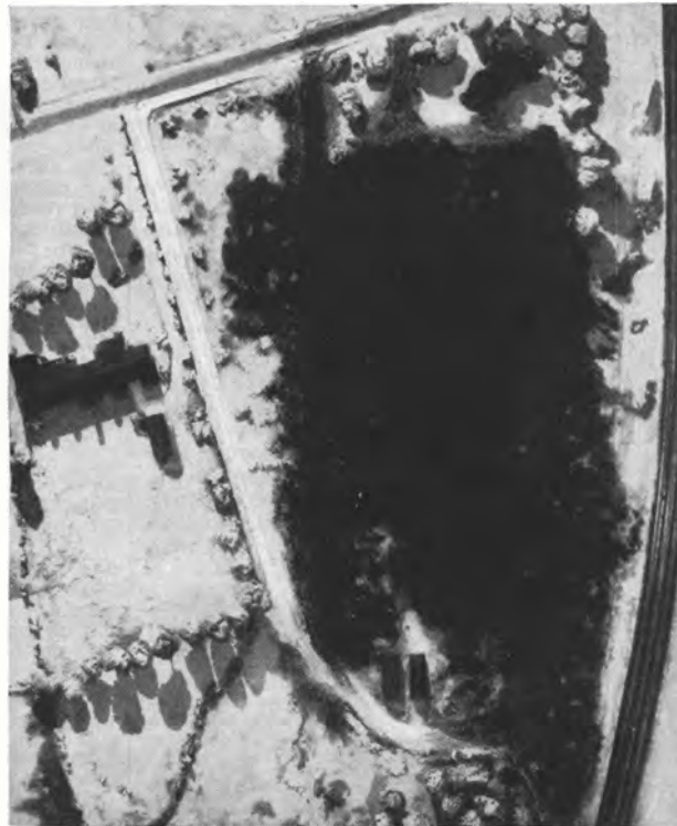
BUT HERE IT IS AGAIN. With Kodak Infrared Film in the aerial cameras, pictures like this are brought back from an observation flight. On Infrared pictures, the false, “dead” camouflage materials look almost black. The natural landscape is unnaturally light. A trained cameraman, with one look, knows where the bombs should strike.
