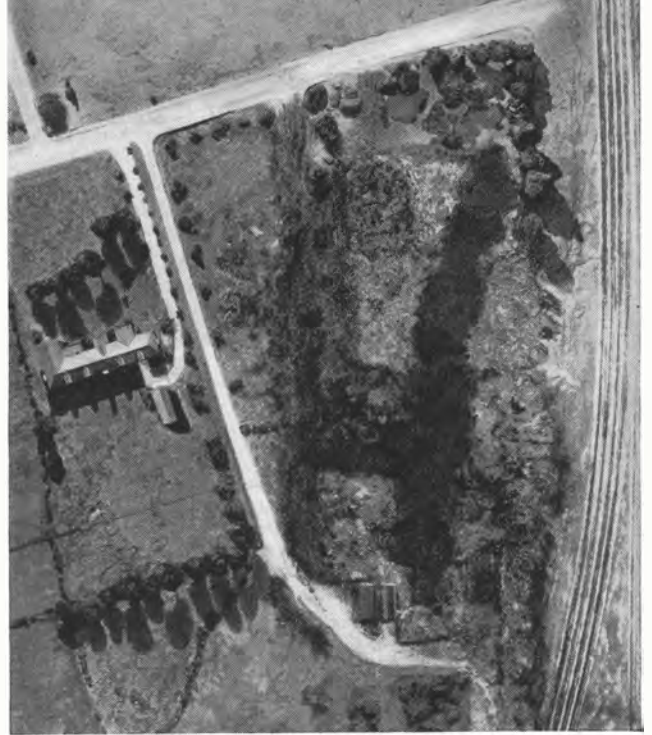
NOW YOU DON'T. With camouflaged materials—false structures, netting, cloth streamers, paint, and artificial trees—the experts have fooled the camera, and the bombardier. To the aerial camera loaded with panchromatic film, even the marks of erosion on the slope by the railroad track have disappeared.
